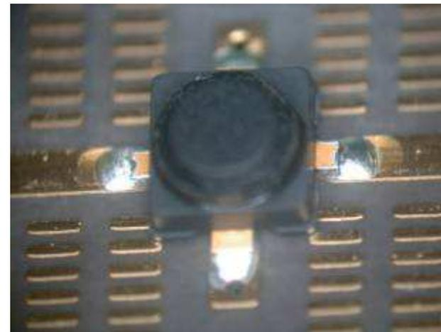
*Fig.1 After reflow in case of the recommended foot pattern*
