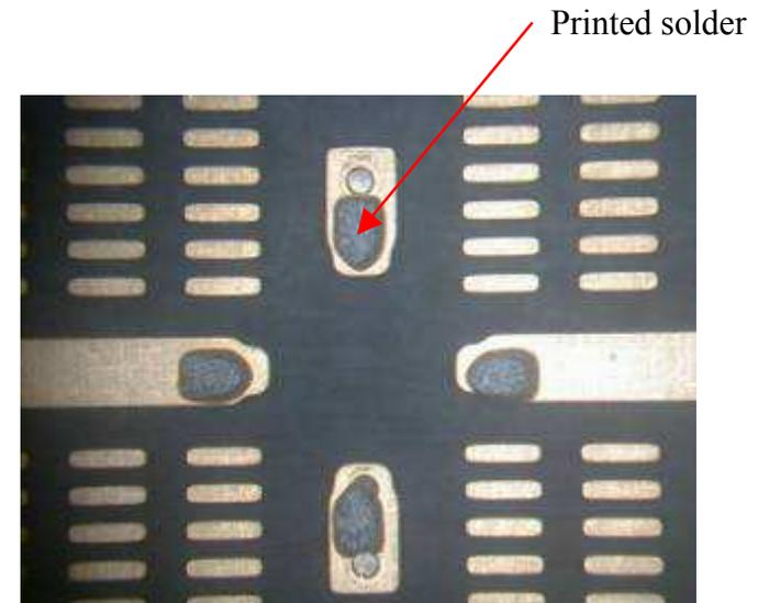
Fig.2 After solder printing
