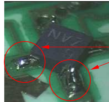
(b) failure mounting
