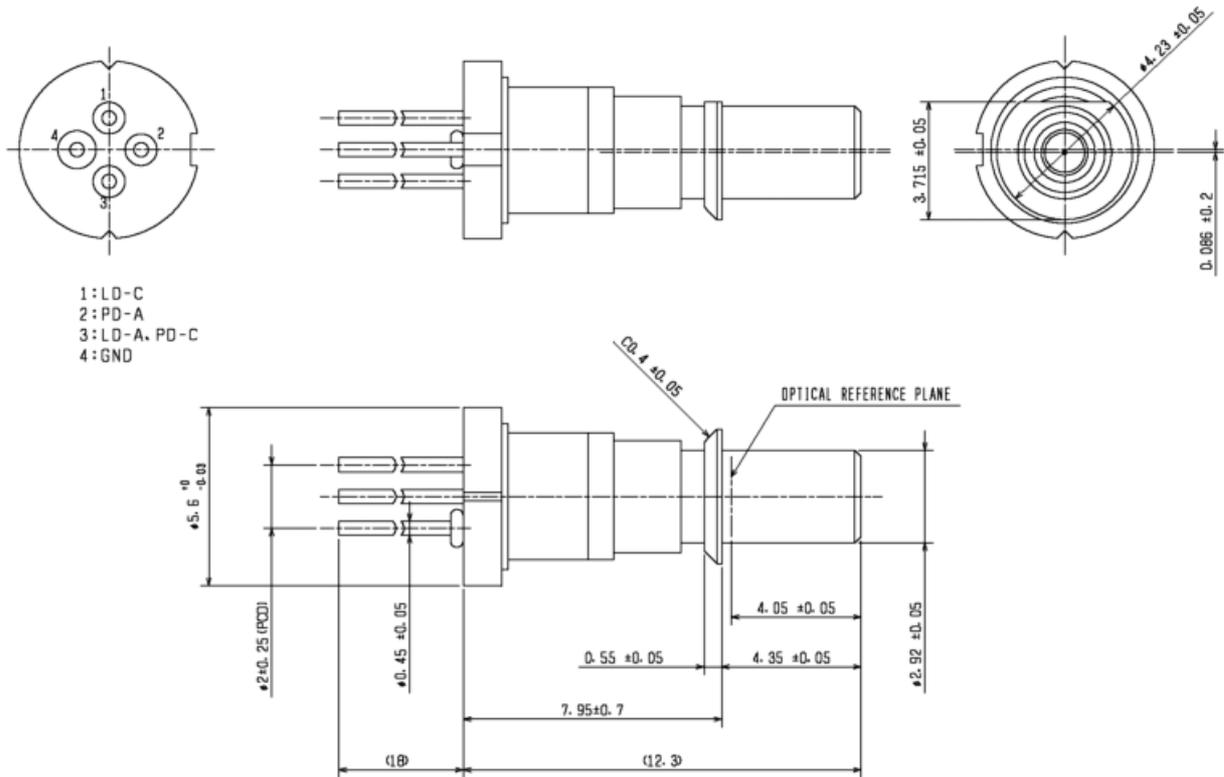
**ES Product****FU-40RDF-S5M2**1.31  $\mu\text{m}$  DFB-LD WITH LC RECEPTACLE FOR LONG HAUL APPLICATIONS**Safety Cautions for Use of Optoelectronic Devices****General:**
