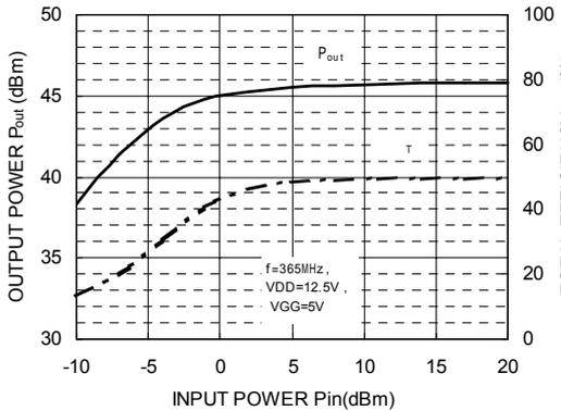
OUTPUT POWER and EFFICIENCY versus INPUT POWER
